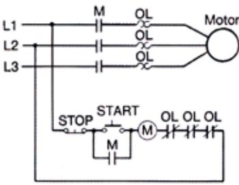
A magnetic starter contains a mechanism for opening and closing a set of contacts in the motor circuit and a thermal overload protective device. When the coil is energized, movable contacts complete the electrical circuit. De-energizing the coil opens the circuit. Magnetic starters are frequently controlled by pushbutton, limit switches, relays, timers, pressure switches, and float switches.
